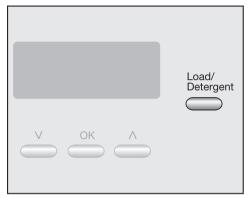
Press and hold the Load/Detergent button pressed in until the following message appears in the display:
